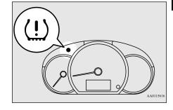
When the ignition switch is turned to the "ON" position, the tyre pressure monitoring system warning lamp normally illuminates and goes off a few seconds later.
