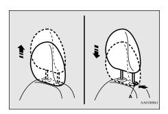
Lift the head restraint with the height adjusting knob (A) pushed in.
