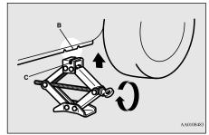
4. Insert the bar (D) into the wheel nut wrench (E). Then put the end of the bar into the shaft's jack end, as shown in the illustration.
