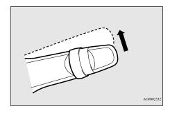
The wipers will operate once if the lever is moved to the "AUTO" position and the knob (C) is turned in the "+" direction when the ignition switch is in the "ON" position or the operation mode is in ON.
