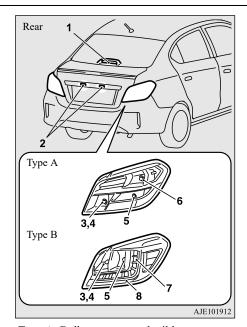
Type A: Bulb type stop and tail lamps Type B: LED type stop and tail lamps
