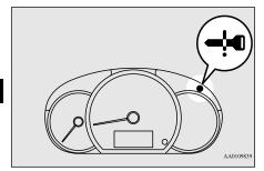
If the operation mode is in OFF and the driver's door is opened with the keyless operation key in the key slot, the warning lamp will blink and the outer buzzer sounds for approximately 3 seconds and the inner buzzer sounds for approximately 1 minute to remind you to remove the key.
