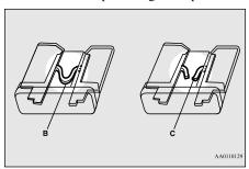
B- Fuse is OK C- Blown fuse
