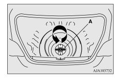
• Put the spare wheel under the vehicle body near the jack. This makes it safer if the jack
