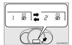
3. The valid tyre ID set is changed, and the number of the tyre pressure monitoring system (TPMS) SET indicator is changed.
